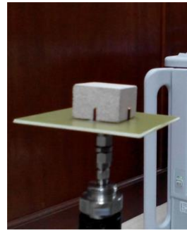
Fig. 1. Pattern reconfigurable dielectric resonator antenna
