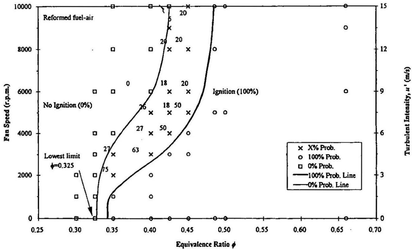
FIGURE 2. Ignition probability for reformed fuel-air mixtures at  $T_u = 328 K$  and  $1 atm$ . Number on graph is percentage of success.
