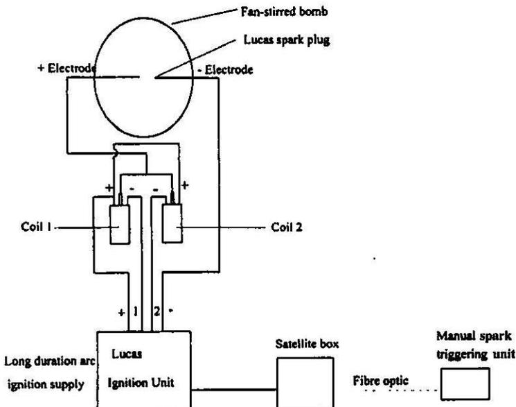
FIGURE 1. Arrangement of ignition probability study apparatus
