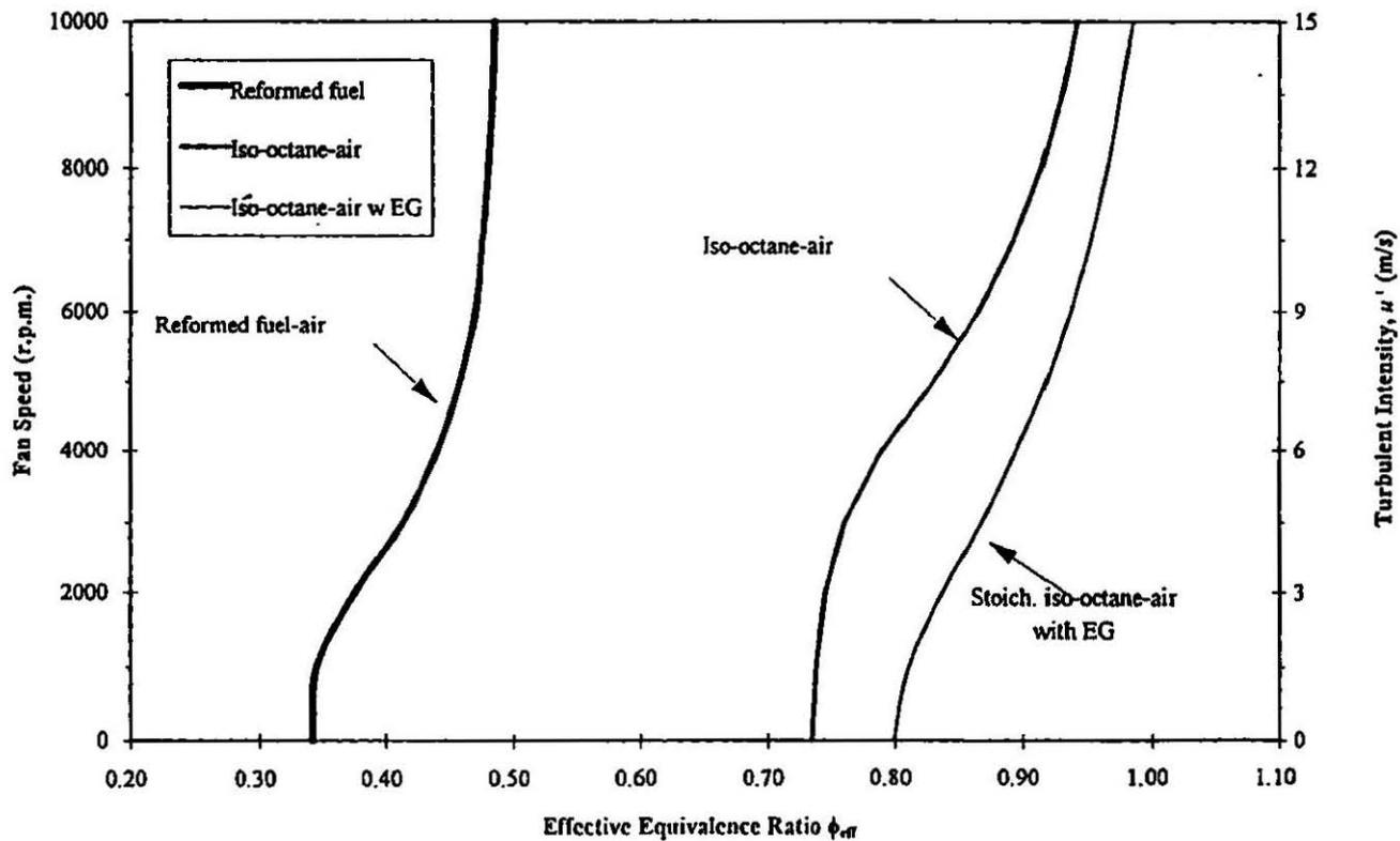
FIGURE 5. Comparison of 100% ignition probability curves for reformed fuel-air, iso-octane-air iso-octane-air with EG at  $T_u = 328 K$  and  $1 atm$ .
