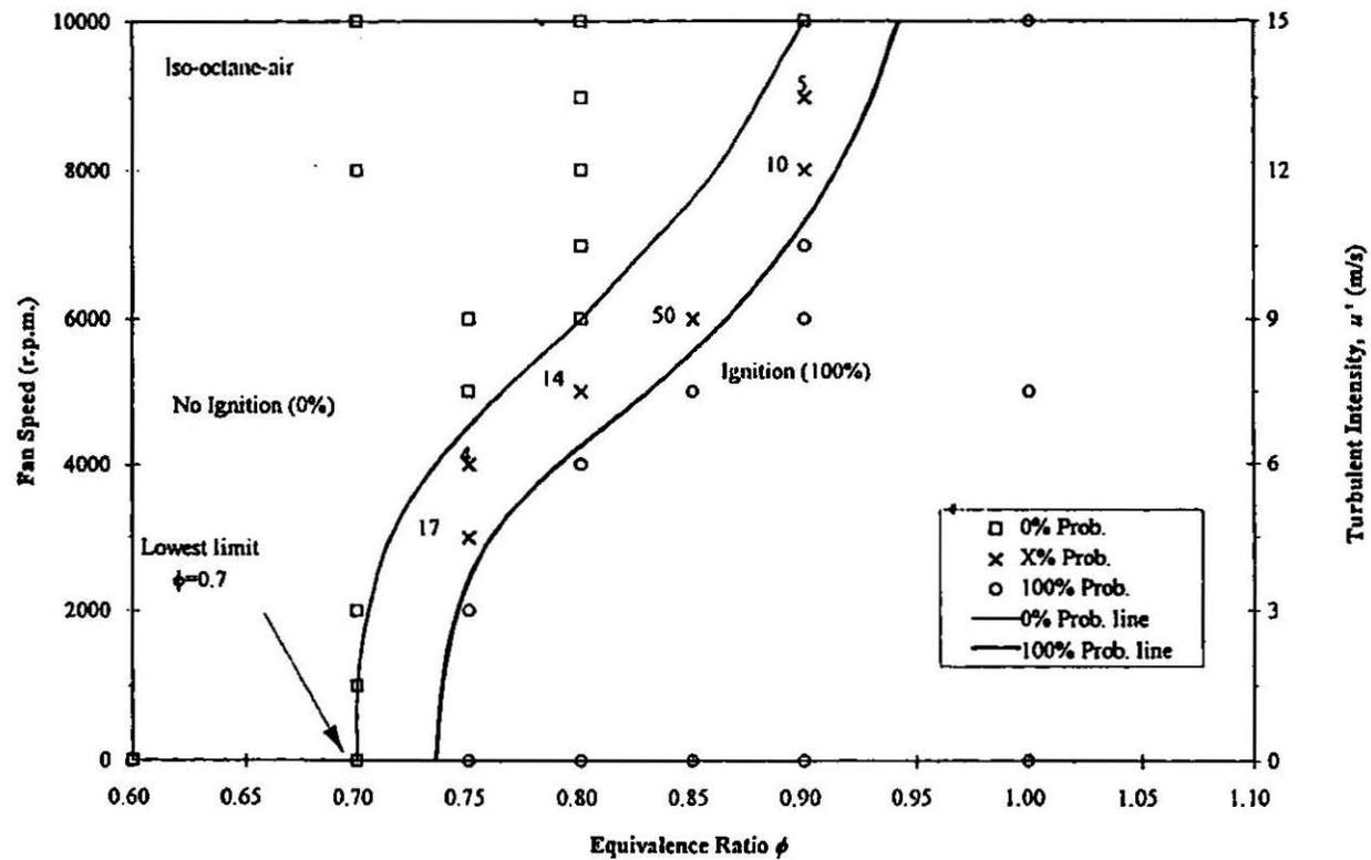
FIGURE 3. Ignition probability for iso-octane-air mixtures at  $T_u = 328\text{ K}$  and  $1\text{ atm}$ . Number on graph is percentage of success.
