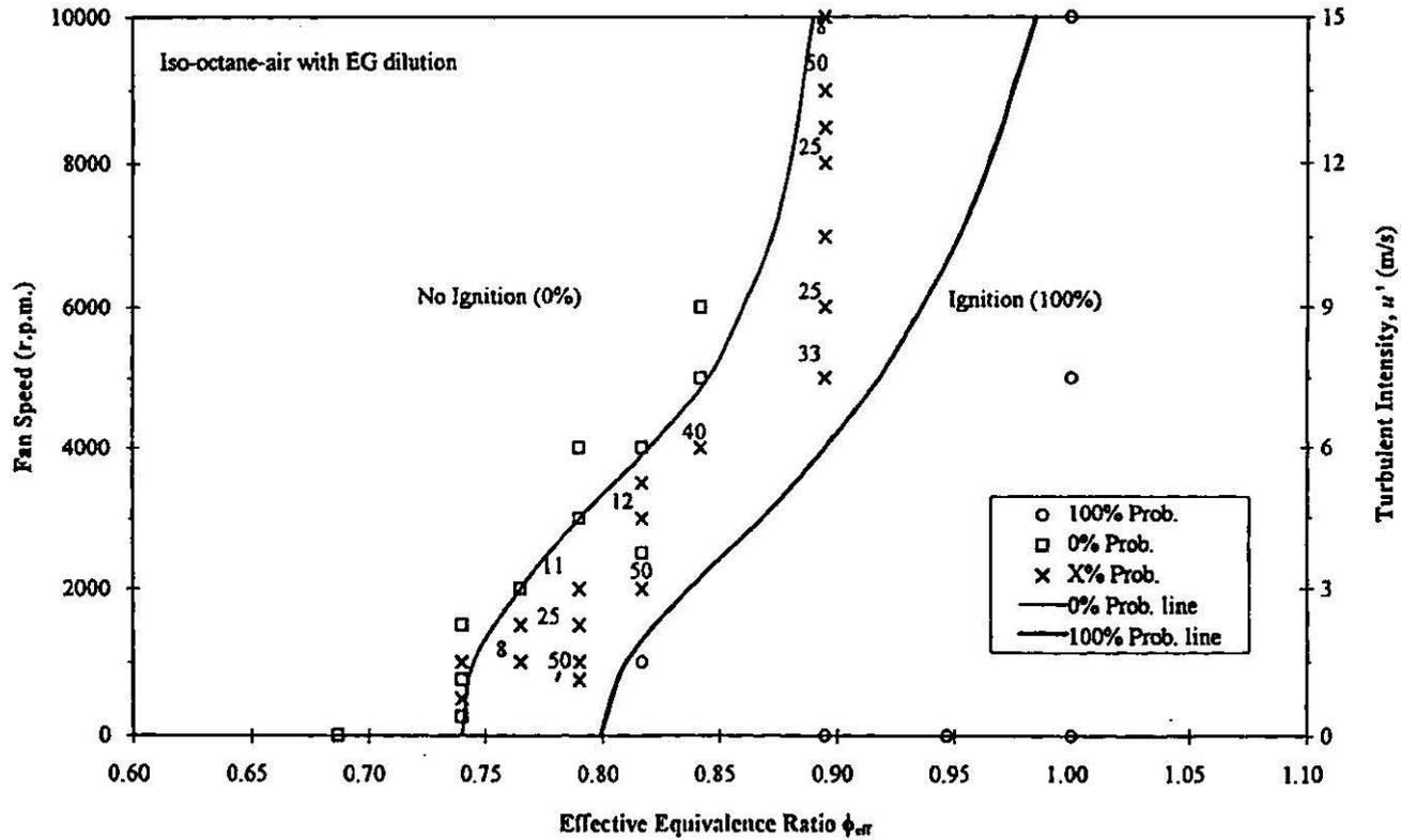
FIGURE 4. Ignition probability for stoichiometric iso-octane-air mixtures with EG at  $T_u = 328 K$  and  $1 atm$ . Number on graph is percentage of success.
