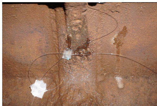
FIGURE 3. FBG sensors with rectangular rosette arrangement at thermite area
