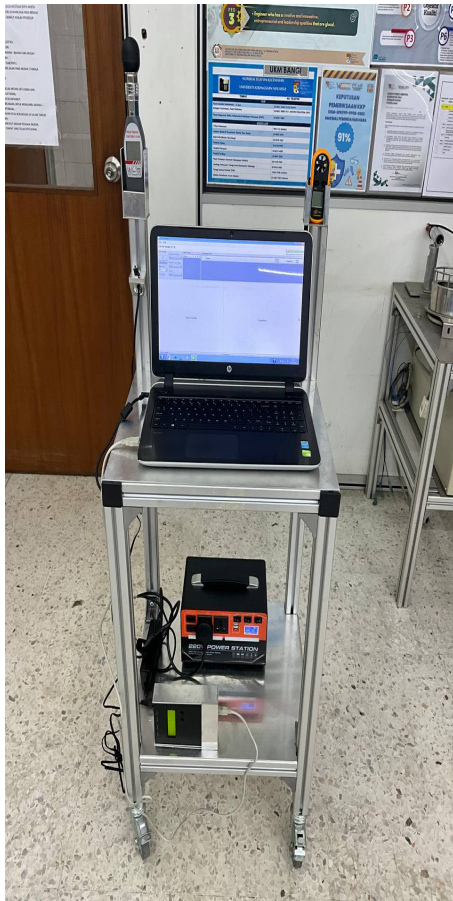
FIGURE 4. Thermal Comfort Station (TCS) to assess UHI and TC
