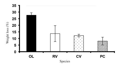
FIGURE 2. Weight loss of kenaf treated with four species of fungi. A total of four flasks were prepared for each species and fungal treatment was repeated three times. Weight loss was averaged among all the replications. OL-Oxyporus latemarginatus, RV-Rigidoporus vinctus, PC-Phanerochaete chrysosporium, CV-Coriolus versicolor
