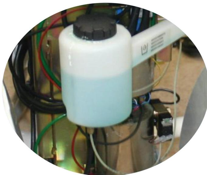
FIGURE 2. Separate bottle for the disinfectant
