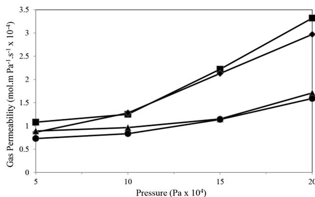
FIGURE 4. Gas permeability of TiO<sub>2</sub> hollow fiber membrane at different ceramic loading and sintering temperature (■) 20 wt. % ceramic loading sintered at 1200°C, (◆) 20 wt. % ceramic loading sintered at 1300°C, (▲) 23 wt. % ceramic loading sintered at 1200°C and (●) 23 wt. % ceramic loading sintered at 1300°C
