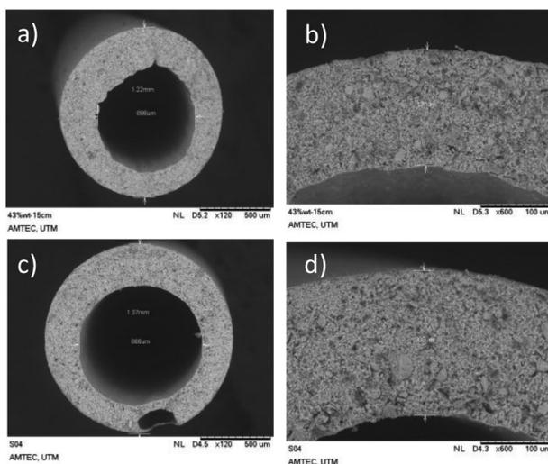
FIGURE 2. Cross-sectional images of TiO<sub>2</sub> hollow fiber membrane prepared from ceramic suspension using mixture of nano-size particles a) 43 wt. % ceramic loading, b) higher magnification of 43 wt. % ceramic loading, c) 45 wt. % ceramic loading and d) higher magnification of 45 wt. % ceramic loading
