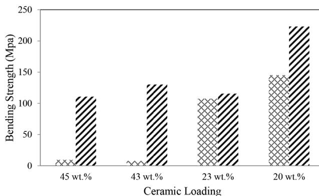
FIGURE 3. Bending strength of TiO<sub>2</sub> hollow fiber membrane for single nano-sized and mixture nano-sized particles sintered at (⊗) 1200°C and (▨) 1300°C
