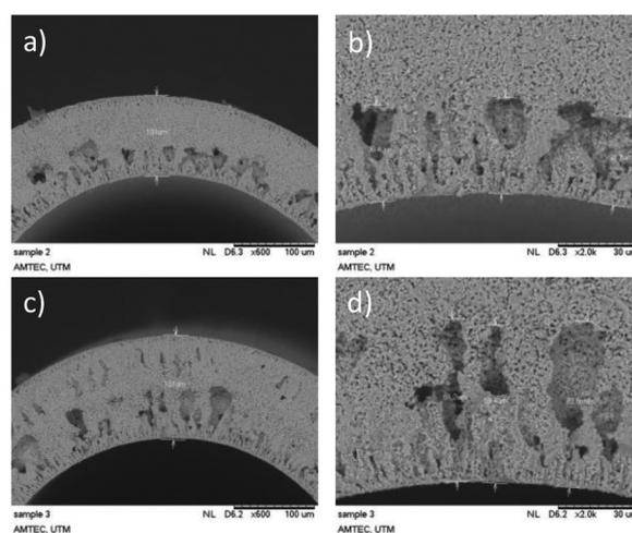
FIGURE 1. Cross-sectional images of TiO<sub>2</sub> hollow fiber membrane prepared from 20 wt. % ceramic suspension using single nano-size particle a) 9 cm air gap length, b) finger-like structure for 9 cm air gap length, c) 12 cm air gap length and d) finger-like structure for 12 cm air gap length
