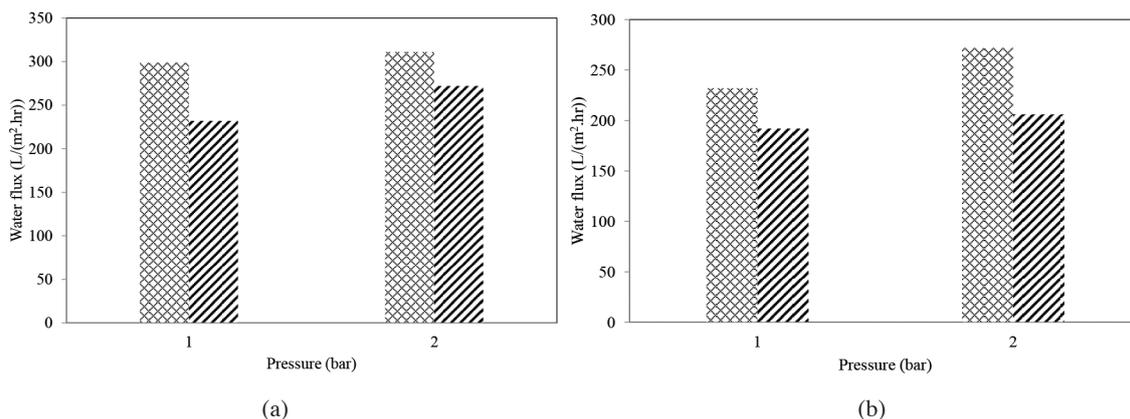
FIGURE 5. a) Water permeation data of  $\text{TiO}_2$  hollow fiber membrane prepared using a mixture nano-size particles at ceramic loading of ( ) 43 wt. % and ( ) 45 wt. % and b) Water permeation data of  $\text{TiO}_2$  hollow fiber membrane prepared using a mixture nano-size particles sintered at ( ) 1200°C and ( ) 1300°C
