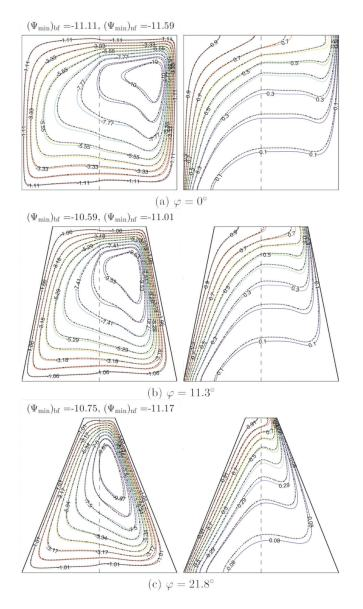
FIGURE 4. Streamlines (left) and isotherms (right) evolution by the side wall inclination angle for  $Ra = 10^5$ ,  $Da = 10^{-3}$ , S = 0.5,  $\varpi = 0^{\circ}$ ,  $\phi = 0$  (solid lines) and  $\phi = 0.05$  (dashed lines)
