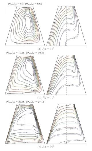
FIGURE 2. Streamlines (left) and isotherms (right) evolution by Rayleigh number for  $Da = 10^{-4}$ , S = 0.5,  $\varphi = 16.7^{\circ}$ ,  $\varpi = 0^{\circ}$ ,  $\phi = 0$  (solid lines) and  $\phi = 0.05$  (dashed lines)
