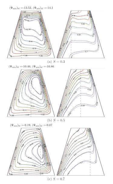
FIGURE 3. Streamlines (left) and isotherms (right) evolution by porous layer thickness for  $Ra = 10^6$ ,  $Da = 10^{-4}$ ,  $\varphi = 16.7^\circ$ ,  $\varpi = 0^\circ$ ,  $\phi = 0$  (solid lines) and  $\phi = 0.05$  (dashed lines)
