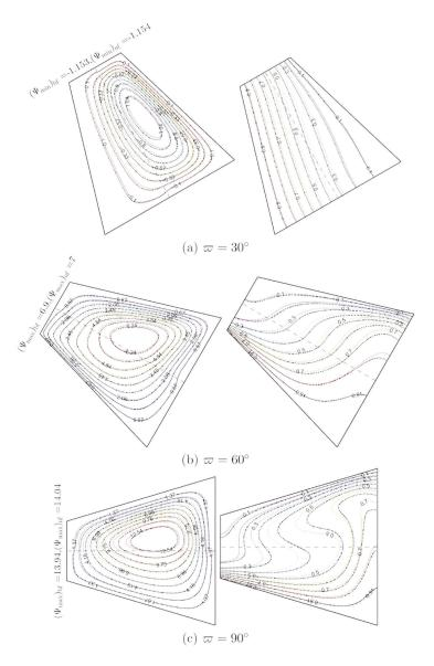
FIGURE 5. Streamlines (left) and isotherms (right) evolution by the inclination angle of the cavity for  $Ra = 10^5$ ,  $Da = 10^{-3}$ , S = 0.5,  $\varphi = 16.7^{\circ}$ ,  $\phi = 0$  (solid lines) and  $\phi = 0.05$  (dashed lines)
