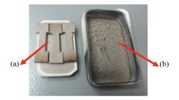
FIGURE 7. Physical deformation after sintering temperature at1100°C (a)Ti-6Al-4V/HA withNaCl(b)Ti-6Al-4V/HA withPMMA
