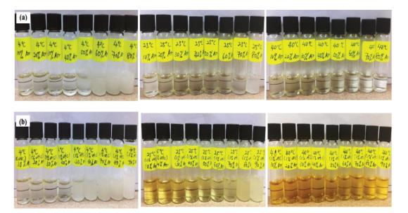
FIGURE 5. Microemulsions stability at 4°C, 25°C and 40°C for (a) basic microemulsions, (b) vitamin C-loaded microemulsions
