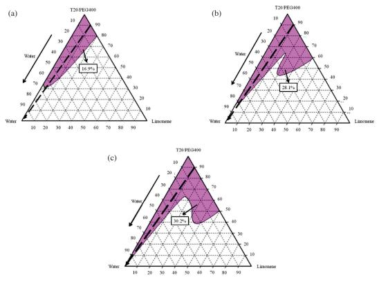
$\label{eq:FIGURE 3. Pseudo-ternary phase diagrams of tween 20/polyethylene glycol 400/limonene/water at (a) Km=1:1, (b) Km=2:1, (c) Km=3:1$
