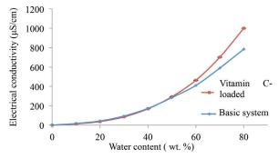
FIGURE 6. Electrical conductivity of basic and system with an addition of vitamin C
