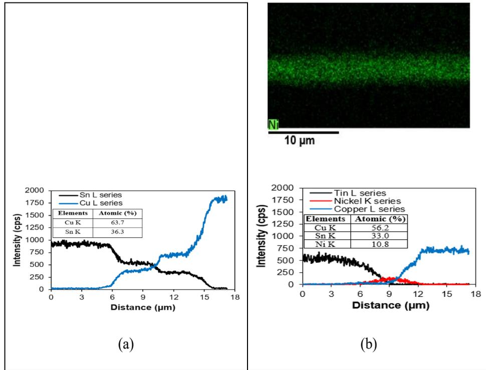
FIGURE 2. EDS analysis of interfacial intermetallic layer of Sn-0.3Ag-0.7Cu solder joint on PCB/Cu with: (a) Sn, and (b) Ni coating subjected to aging for 1000 h
