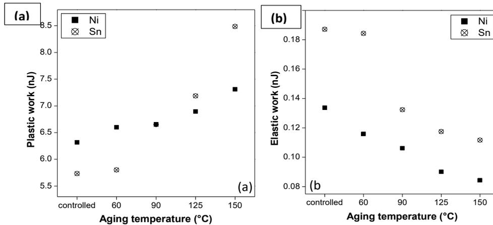
FIGURE 7. (a) Plastic, and (b) elastic work properties of Sn-0.3Ag-0.7Cu solder joint on PCB with different coating subjected to aging for 1000 h
