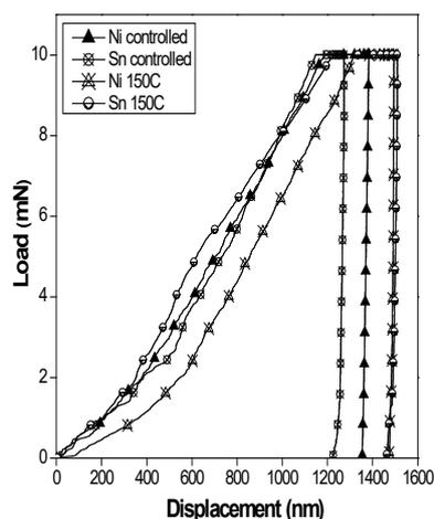
FIGURE 4. Load displacement curve of Sn-0.3Ag-0.7Cu solder joint on PCB/Cu with different coating subjected to aging at 150°C for 1000 h
