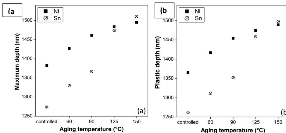
FIGURE 5. (a) Maximum, and (b) plastic depth properties of Sn-0.3Ag-0.7Cu solder joint on PCB with different coating subjected to aging for 1000 h
