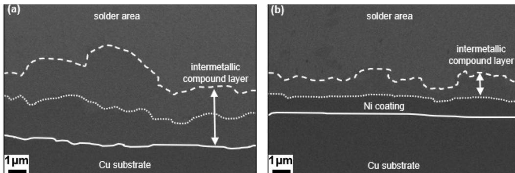
FIGURE 1. FESEM Micrograph of Sn-0.3Ag-0.7Cu solder joint on PCB/Cu with: (a) Sn, and (b) Ni coating after aging at 150 °C for 1000 h
