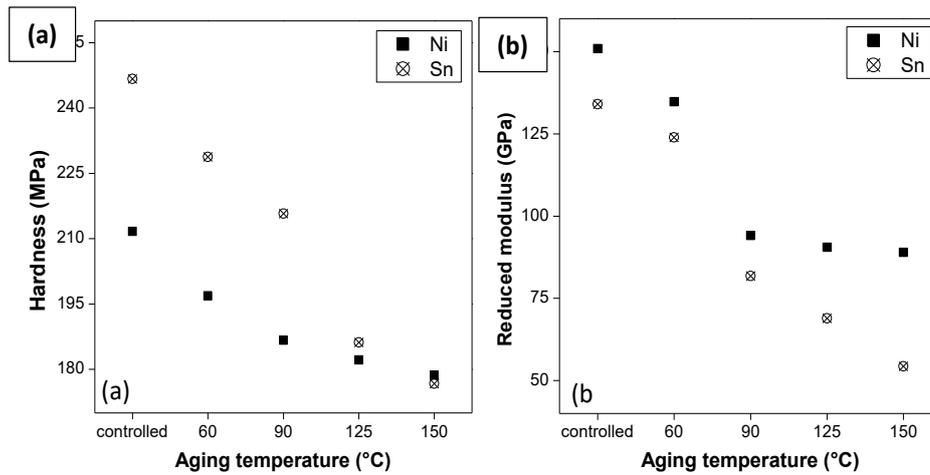
FIGURE 6. (a) Hardness, and (b) reduced modulus properties of Sn-0.3Ag-0.7Cu solder joint on PCB with different coating subjected to aging for 1000 h
