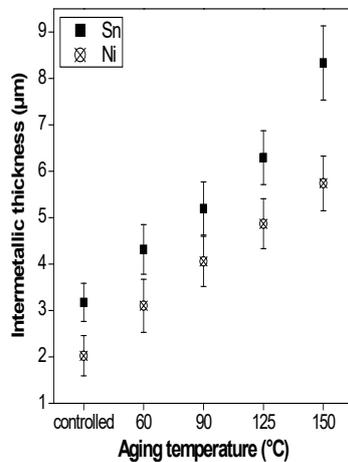
FIGURE 3. Intermetallic thickness of Sn-0.3Ag-0.7Cu solder joint on PCB/Cu with different coating subjected to aging for 1000 h
