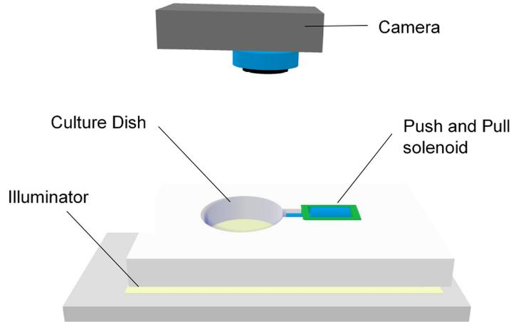
FIGURE 1. Setup for startle habituation assay. The startle apparatus consists of a single swim arena with a solenoid attached at the side to produce sudden taps
