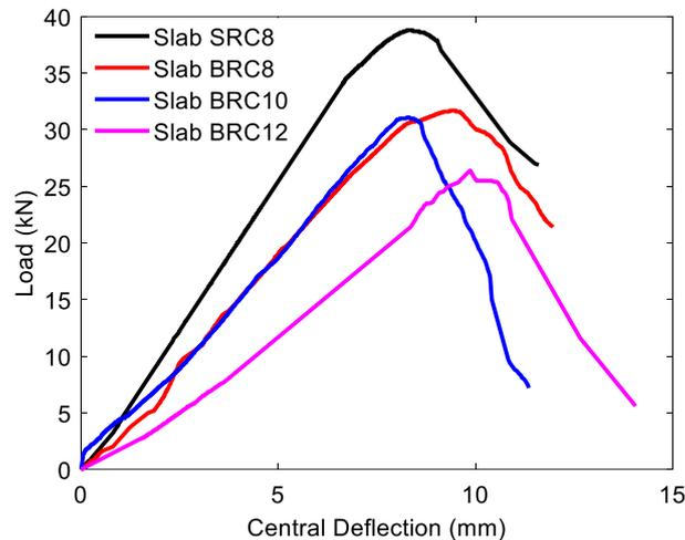
FIGURE 5. Load-deflection characteristics of tested slabs
