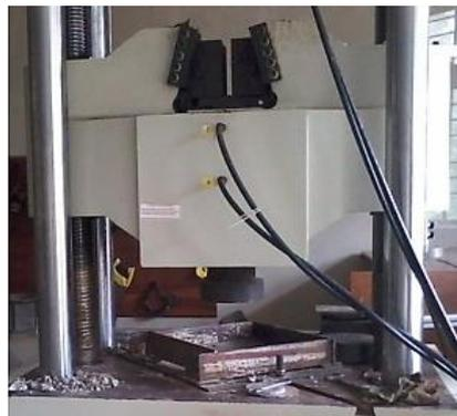
a) Universal Testing Machine (UTM) for slab test
