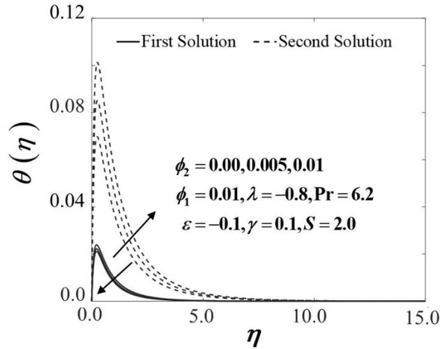
FIGURE 5.  $\theta(\eta)$  along the shrinking cylinder ( $\lambda = -0.8$ )
