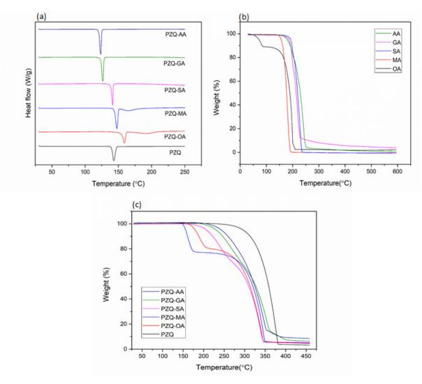
FIGURE 4. DSC thermograms of pure PZQ and its co-crystals (a), TGA thermograms of co-crystal formers (b), TGA thermograms of PZQ and its co-crystals (c)
