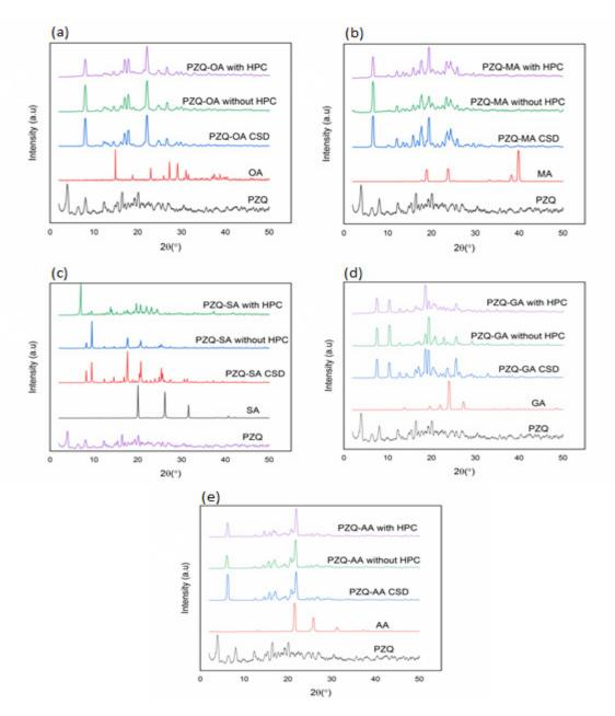
FIGURE 2. XRPD patterns of pure PZQ, respective co-crystal formers, and cocrystals with/without HPC polymer
