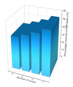
FIGURE 6. The reusability of LNR/AAc hydrogel for MB adsorption
