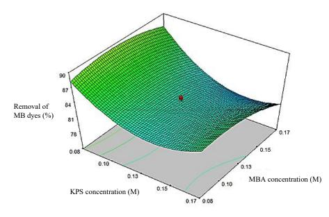
FIGURE 5. Response surface interaction between parameters KPS concentration and MBA concentration
