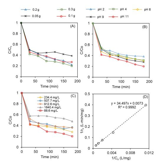
FIGURE 5. Parameter studies of 0.005Ag-0.005Ce-ZnO photocatalysis (A) effect of catalyst loading, (B) effect of initial pH, (C) effect of TCE concentration, and (D) Langmuir-Hinshelwood linear plot (experimental conditions: 88.6-1640.4 mg TCE/L, 0.05-0.3 g catalyst/100 mL, and initial pH 2-11)
