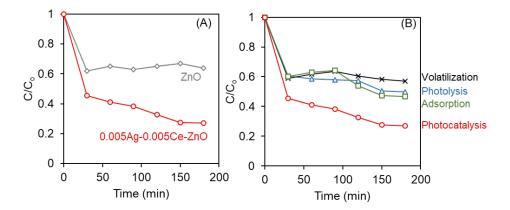
FIGURE 4. (A) Photocatalytic performance of ZnO and 0.005Ag-0.005Ce-ZnO under visible light and (B) control experiments of 0.005Ag-0.005Ce-ZnO (experimental conditions: 100 mg TCE/L, 1 g catalyst/L, and pH 6)
