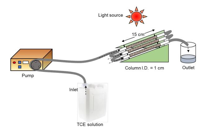
FIGURE 1. Fixed bed photoreactor setup for continuous flow treatment of TCE over 0.005Ag-0.005Ce-ZnO@Al,O<sub>3</sub>
