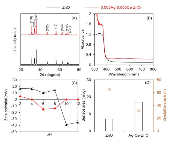
FIGURE 2. Characterization of ZnO and 0.005Ag-0.005Ce-ZnO, (A) XRD profiles, (B) UV-DR, (C) zeta potentiometry, and (D) BET specific surface area calculated from N, adsorption-desorption and crystallite size calculated from XRD patterns
