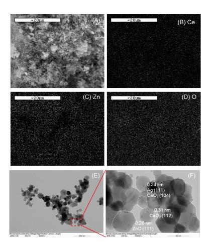
FIGURE 3. (A) SEM image of 0.005Ag-0.005Ce-ZnO with elemental mapping of (B) Ce, (C) Zn, and (D) O, and (E-F) TEM images
