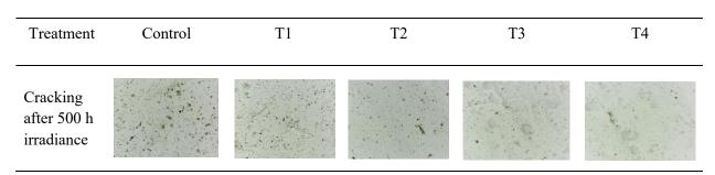
FIGURE 3. Cracking. After 500 h of irradiance, the Control Group (first figure from left) showed a regular pattern of adhesion, whereas all other treatment patterns were irregular (ASTM D610). A Digital Microscope 1600X, Canon Vixia HF R600 32× Optical zoom was used for observations
