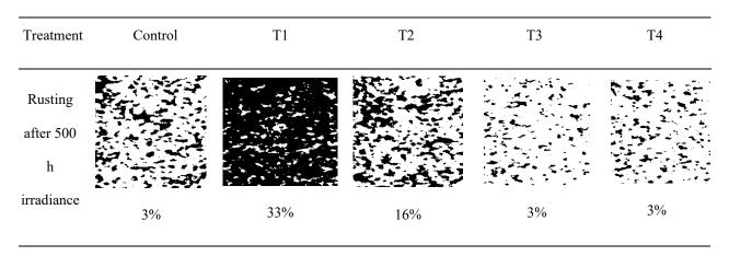
FIGURE 4. Degree of rusting for control group and treatments. A Digital Microscope 1600X, Canon Vixia HF R600 32× Optical zoom was used for observations
