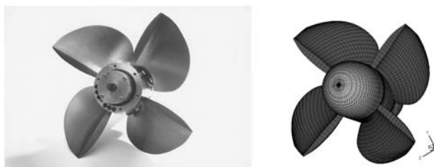
Fig. 9.23. Propeller model 841-B from Olofsson 56 with the corresponding BEM model on the right (from Young & Kinnas 54 ).
