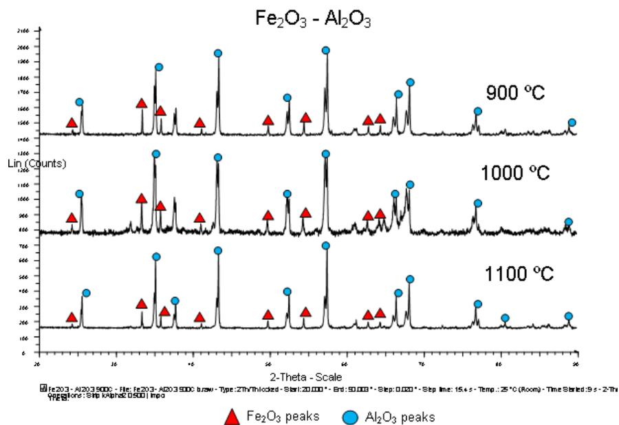
Figure 4. Diffractograms for alumina supported iron (III) oxide (Fe<sub>2</sub>O<sub>3</sub>) catalyst with calcination temperatures of (a) 900 °C, (b) 1000 °C and (c) 1100 °C
