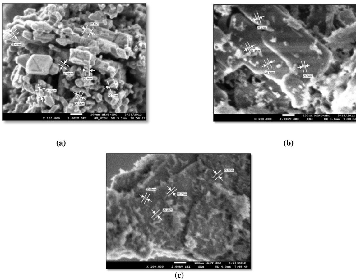
Figure 6. The FESEM micrographs with 100,000 magnifications of (a) CuO/Al<sub>2</sub>O<sub>3</sub> (b) Fe<sub>2</sub>O<sub>3</sub>/Al<sub>2</sub>O<sub>3</sub> and (c) ZnO/Al<sub>2</sub>O<sub>3</sub> calcined at 1000 °C for 5 hours. Scale bar: 100nm.
