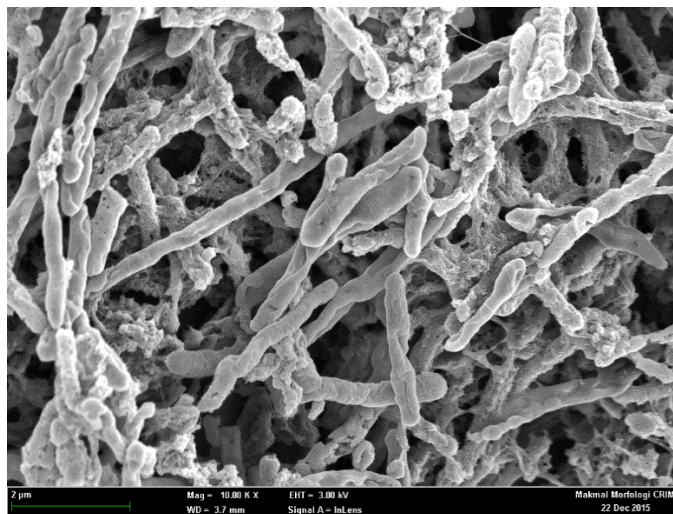
Figure 4(b). FESEM image of attached cell on micro-pores GAC in the cultural medium at 10.00k x magnification
