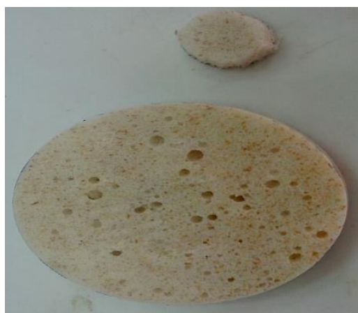
Figure 2. Polymer foam composites prepared for sound absorption coefficient measurement using impedance tube testing
