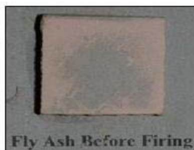
Figure 5. Fly Ash Glaze before firing Figure 6. Fly Ash Glaze after firing
