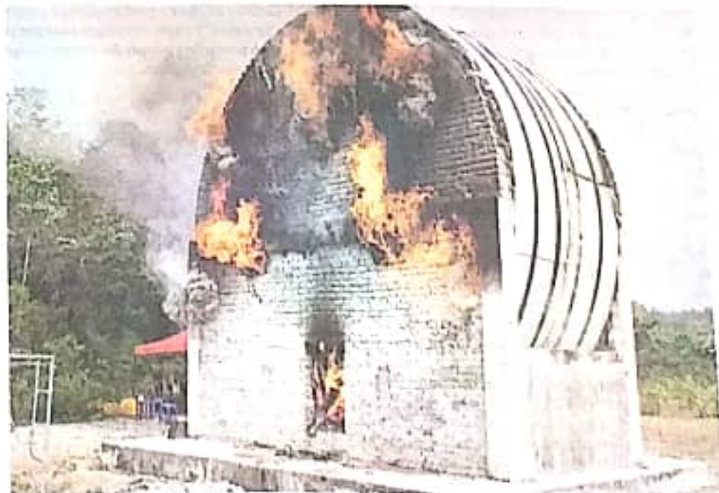
A large scale fire testing of the concrete tunnel lining being carried out at the Fire Research Centre in Bandar Enstek, Negeri Sembilan. PIC COURTESY OF UKM
