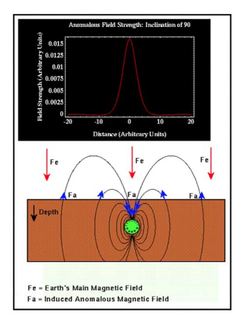
At the north (magnetic) pole, the Earth's main magnetic field, Fe, points straight down. Because the buried sphere is composed of a material with a non-zero <u>susceptibility</u>, the Earth's main magnetic field causes the sphere to produce an <u>induced</u> magnetic field. Field lines associated with this induced field are shown by black lines, and the magnitude and direction of the induced, anomalous field, Fai, at the surface of the earth are shown by the blue arrows.
