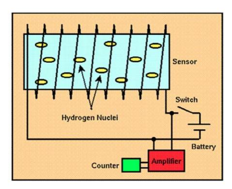
The sensor component of the proton precession magnetometer is a cylindrical container filled with a liquid rich in hydrogen atoms surrounded by a coil. Commonly used liquids
