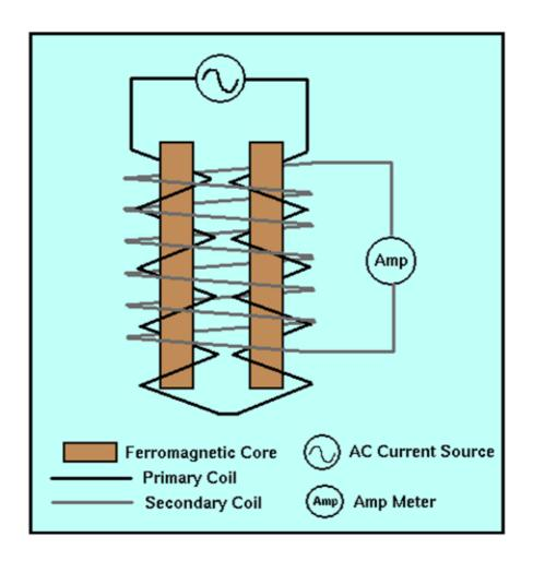
The fluxgate magnetometer is based on what is referred to as the *magnetic saturation circuit*. Two parallel bars of a <u>ferromagnetic</u> material are placed closely together. The <u>susceptibility</u> of the two bars is large enough so that even the Earth's relatively weak magnetic field can produce near *magnetic saturation\** in the bars.
