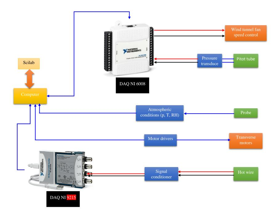
The atmospheric conditions (p, T and RH) were measured using Comet H7331 device. The specs of the device are listed in table 1. The device was connected to the PC via a USB connection. The Modbus protocol was used to transfer data from the apparatus to Scilab. The Modbus module can be loaded on Scilab from the module manager – ATOMS. A simple Scilab code then can be elaborated to get the data from the Comet H7331 registers:
