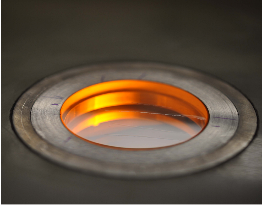
FIGURE 2.7: Equipment for Oil-Film Interferometry: transparent glass plug on wind tunnel wall
