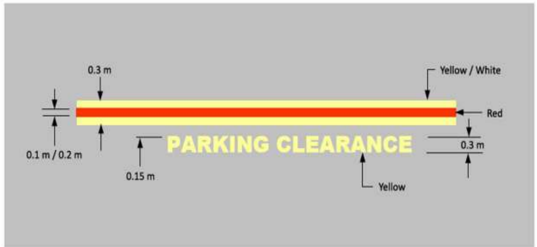
Gambar 5.2-24 : Parking clearance line
