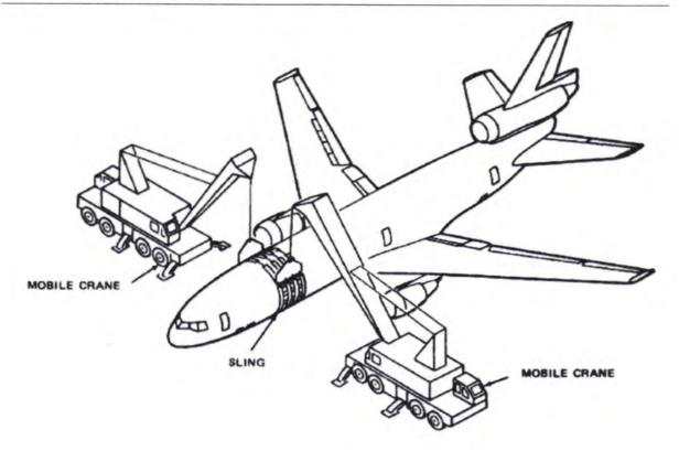
Fig 1-3. Method of lifting nose with mobile cranes from nose down attitude
