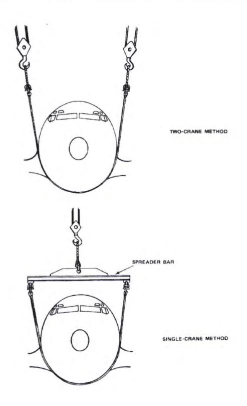
Fig 1-2. Method for lifting nose with mobile cranes from nose down attitude
