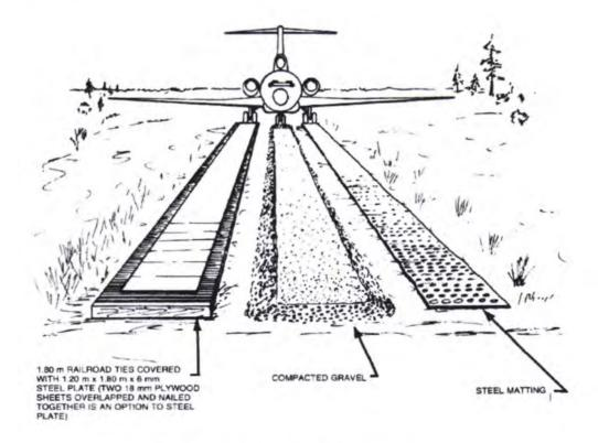
Fig 1-1. Typical prepared surfaces
