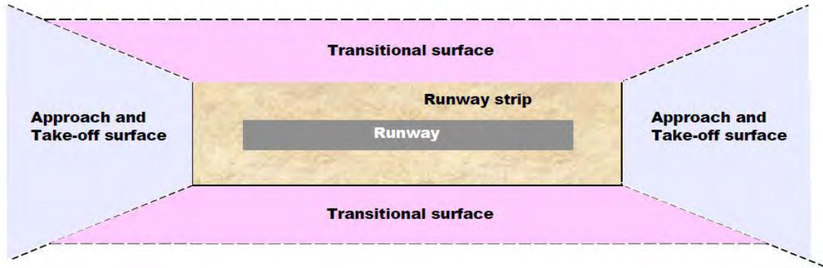
Figure 13.2-1: Obstacle limitation surfaces (inner horizontal surface omitted for clarity)
