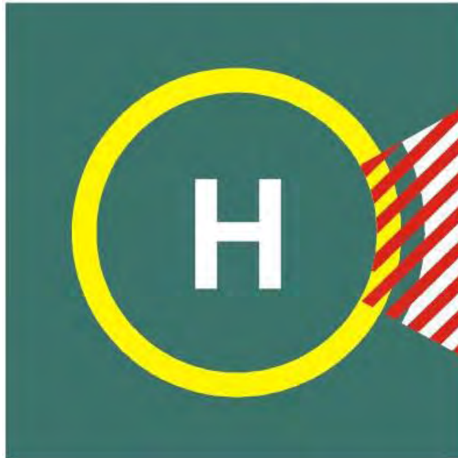
Figure 15-26 Helideck prohibited landing sector marking
