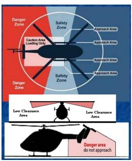
B. The PBC for a helicopter must contain guidance to avoid contact with the main and tail rotors during an emergency evacuation, that will include the possible dipping of the main rotor.
