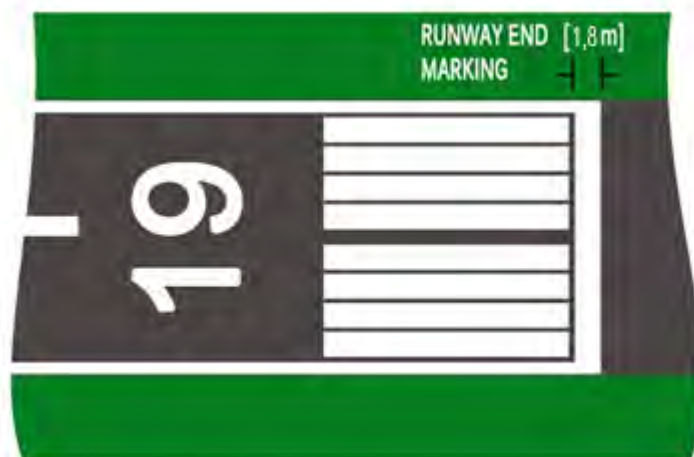
Gambar 8.6-14: Marka Runway End
