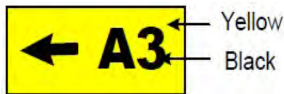
Gambar 8.14-20: Runway exit sign
