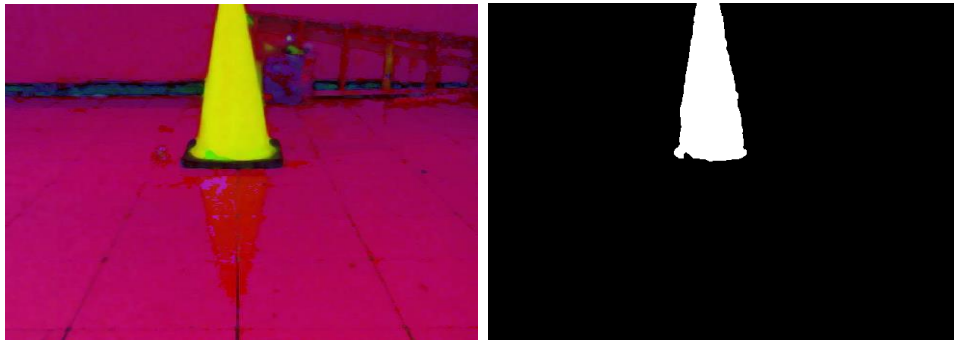
FIGURE 10. Result of the Conversion from HSV image to Binary image
