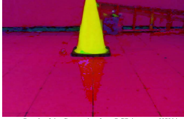
FIGURE 9. Result of the Conversion from RGB image to HSV image
