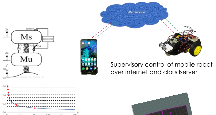
Optimal multiple model adaptive controller design for active vehicle suspensions - suspension model (top) and optimised candidate model selection (bottom)
