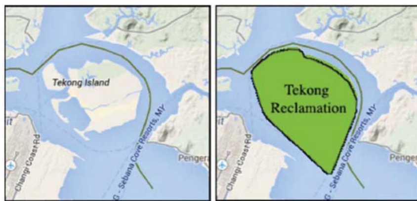
FIGURE 3. Tekong Island: before (left) and after (right) reclamation
