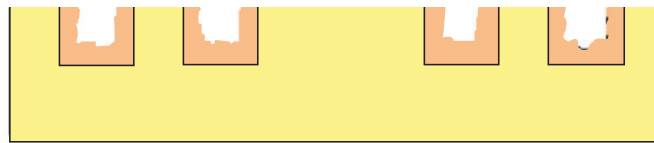
FIGURE 4. Post Tungsten CMP Profile
