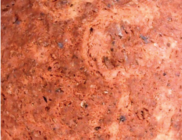
FIGURE 2. The surface texture of LECA
