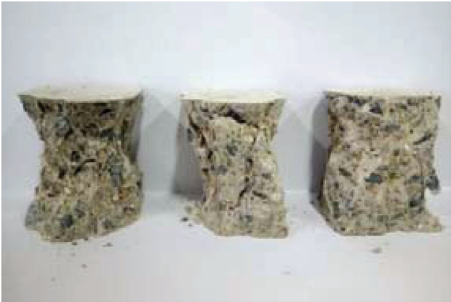
FIGURE 4. The shape failure of NWC
