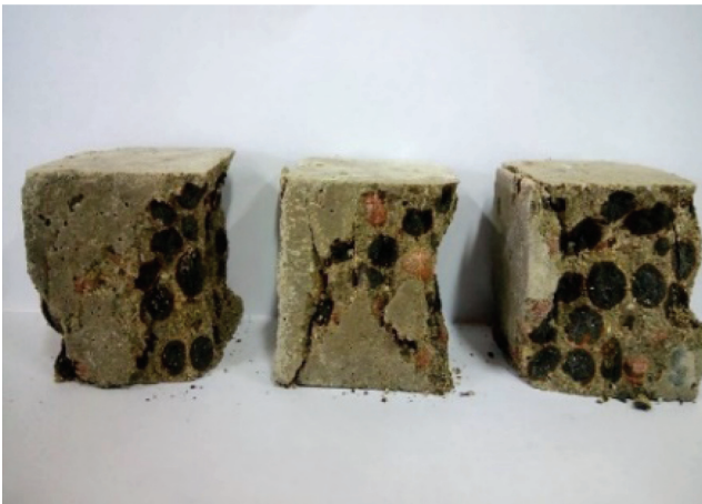
FIGURE 5. The shape failure of LWAC
