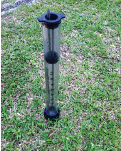
FIGURE 6. Mini-Disk Infiltrometer used to get the infiltration rate
