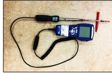
FIGURE 4. The multiparameter ventilation meter
