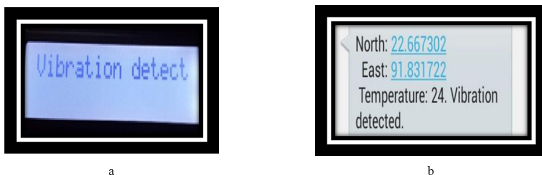
FIGURE 6. Condition of Vibration sensor output (a) Detected condition of vibration (b) Sent message in parent's mobile
