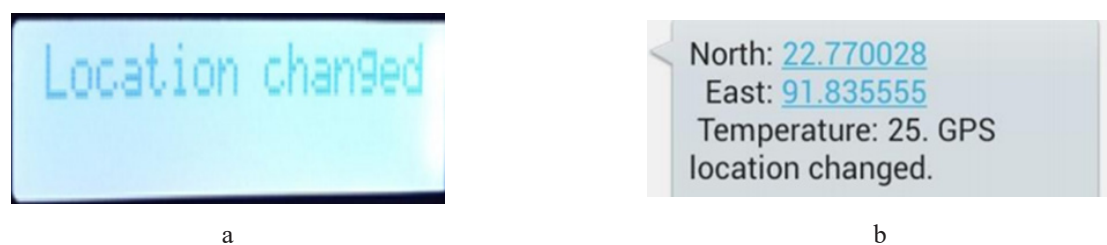
FIGURE 8. Condition of Changed location output (a) shows 'location changed' signal in the display (b) Sent message to the parent's mobile
