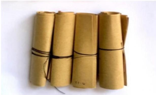
FIGURE 3. The insulating paper being tied before dried
