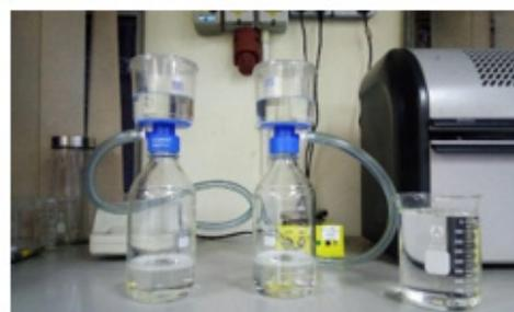
FIGURE 2. Transformer oil filtration
