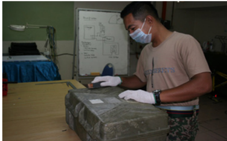
FIGURE 6. Application of sand paper on the E-PPS case
