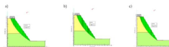
FIGURE 9. Critical slip surface formation for a surcharge load intensity of 14kN/m<sup>2</sup> imposed from a distance of (a) 0 m, (b) 1 m, and (c) 2 m
