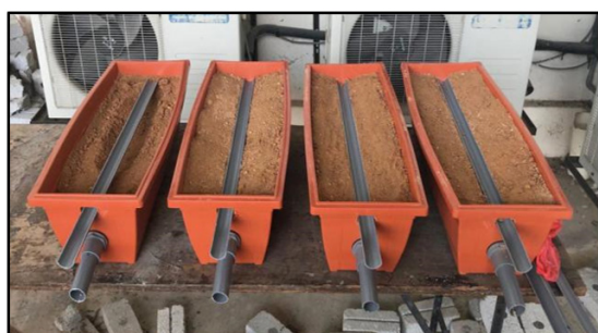
FIGURE 2. Arrangement of pipe as drainage
