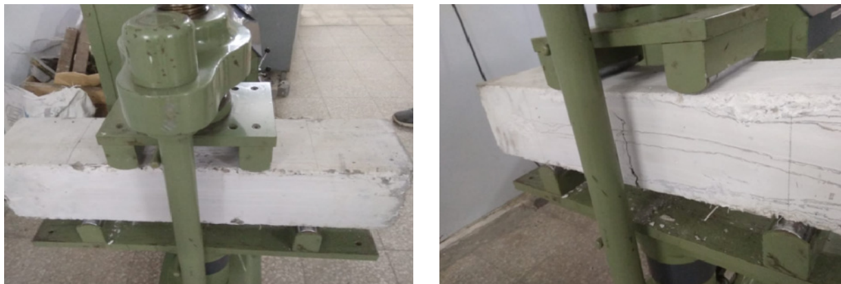
FIGURE 5. Beam specimens under flexure
