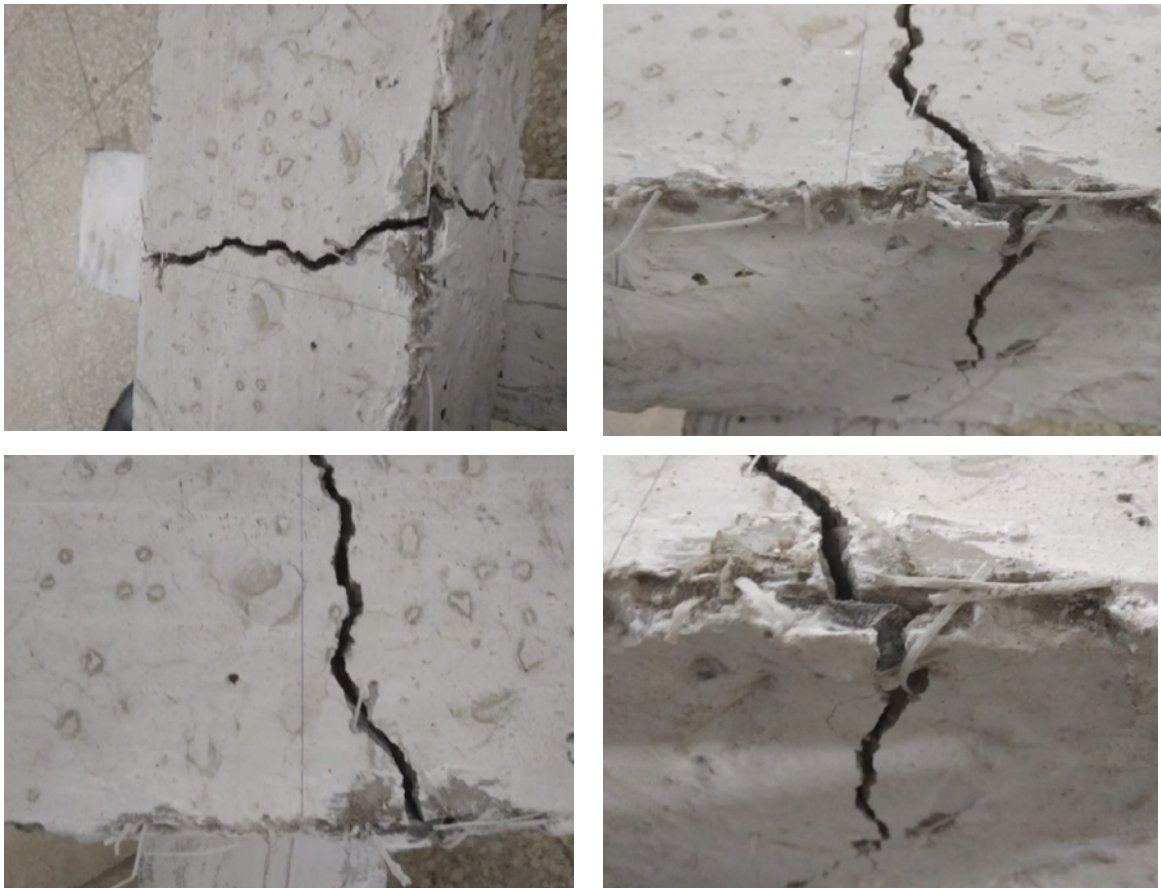
FIGURE 30 Different modes of failure and failure pattern with Polypropylene fibers in higher V_f=0.25
