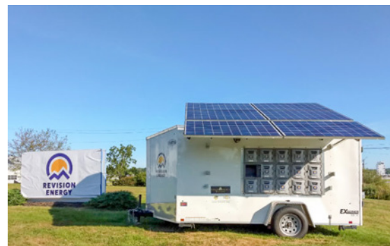
FIGURE 2. Emergency solar trailers for disaster relief (Scribner 2019)
