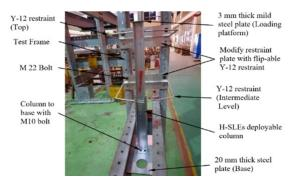
(a) H-SLEs deployable mechanism at vertical configuration
