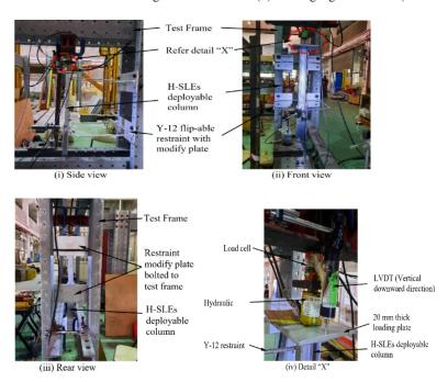
(c)Views of isolated H-SLEs deployable column under load test configuration
