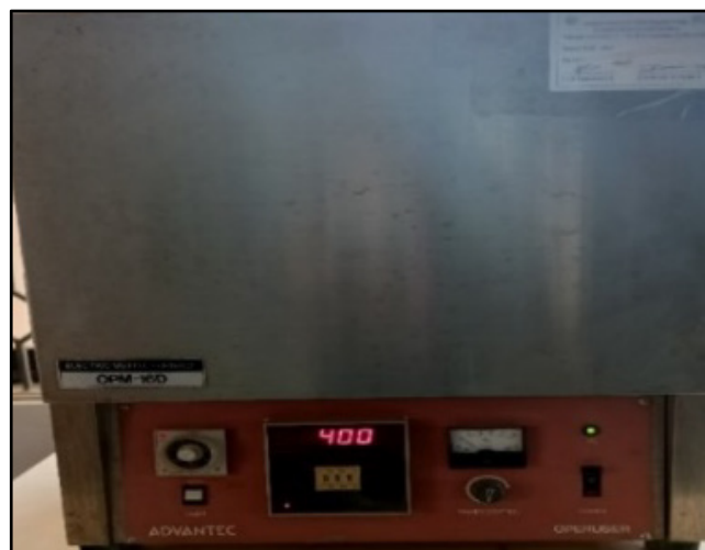
FIGURE 1. Preparation of Buffalo Dung ash in Muffle Furnace
