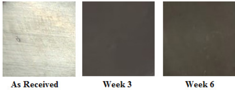
FIGURE 5. Visual Inspection for Pure Aluminium after exposure
