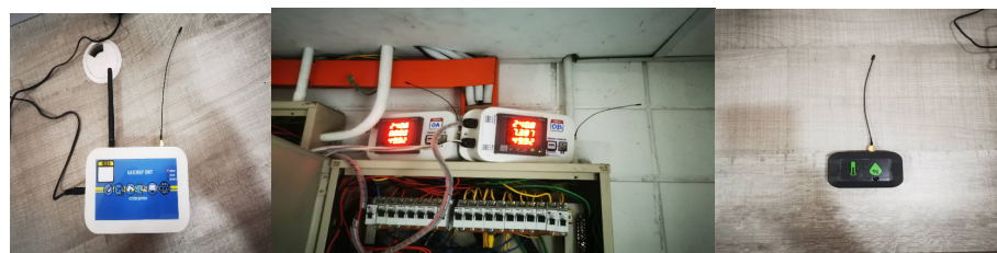
FIGURE 2. (a) Temperature and humidity sensor; (b) Power meter sensors; (c) IoT gateway.
